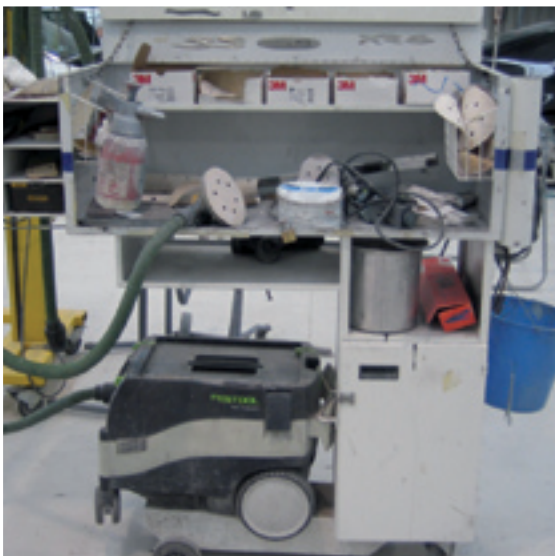
Efficient practices in the sanding area and vacuuming equipment can aid in the capture of polluting dust particles.
