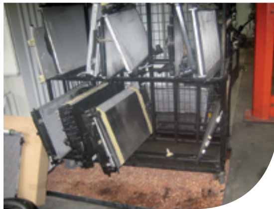
Drip trays are an efficient way of catching leaking radiator coolant.
