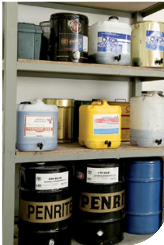
Fitting taps on chemical containers will minimise losses and spillage.
