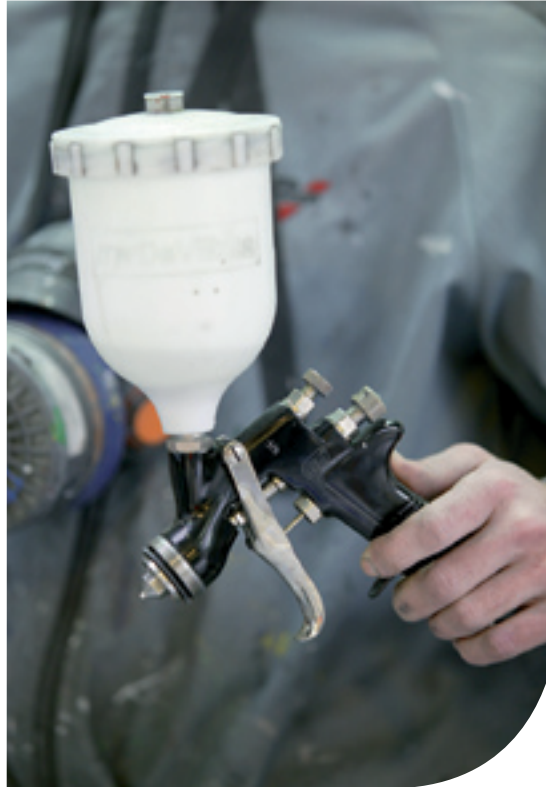
A High-Volume/Low-Pressure (HVLP) spray gun.
