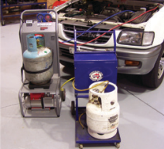
Gas used in vehicle air conditioners can be extracted and recycled.
