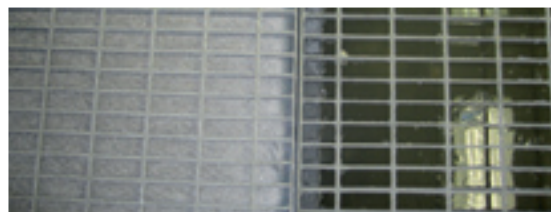
Water and fabric being used in a filter on a spray booth floor.
