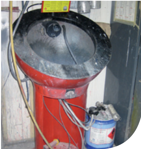
A solvent recycling unit will reduce solvent purchase and disposal costs.
