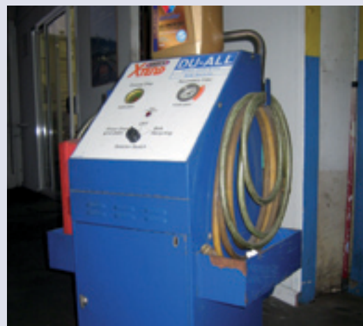
A radiator coolant recycler.
